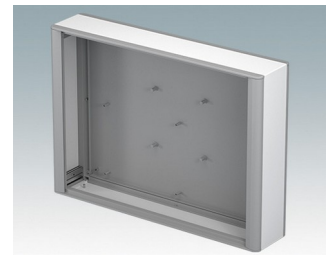
M7042206 TECHNOMET-CONTROL C430V Aluminum Traffic white/traffic gray A RAL 9016/7042 16.54"x11.81"x3.74"
