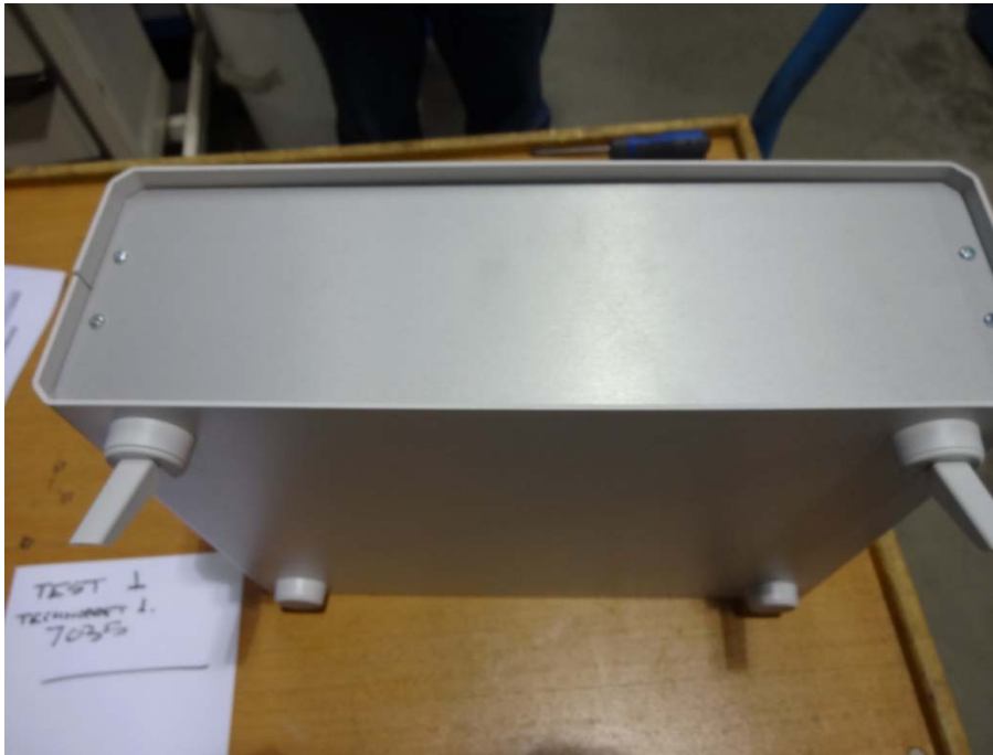
Figure 2.2.1 EUT 1. Enclosure with Technofeet canted ready for topple test
