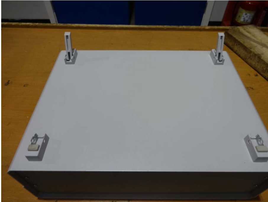
Figure 2.2.7 Post-Test Inspection. EUT 4. Case Feet. No damage observed to the feet or the enclosure
