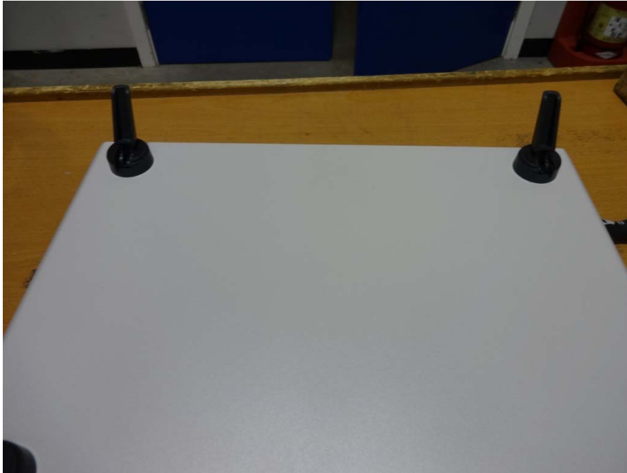
Figure 2.2.5 Post-Test Inspection. EUT 2. Technofeet. No damage observed to the feet or the enclosure
