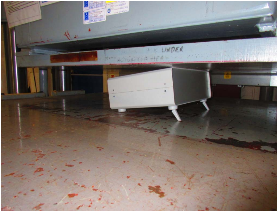
Figure 2.1.1 Enclosure with Technofeet under compression machine platen
