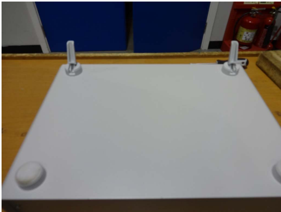
Figure 2.2.4 Post-Retest Inspection. EUT 1. Technofeet. No damage observed to the feet or the enclosure
