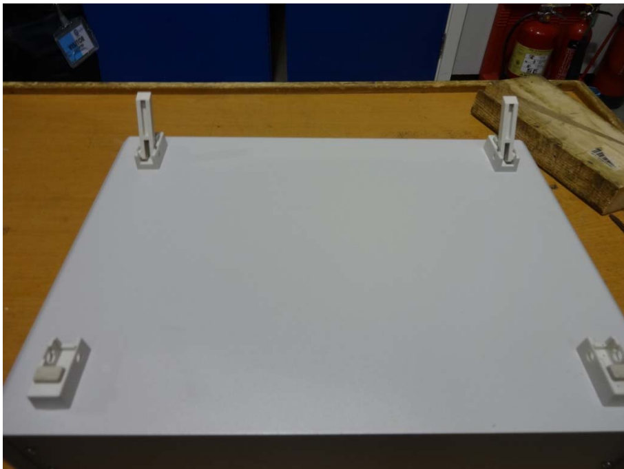
Figure 2.2.8 Post-Test Inspection. EUT 5. Case Feet. No damage observed to the feet or the enclosure
