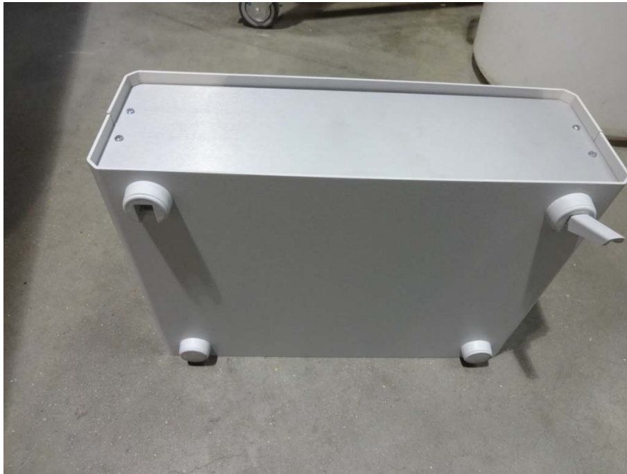
Figure 2.2.3 Post-Test Inspection. EUT 1. Technofeet. One foot (left hand side) unclipped
