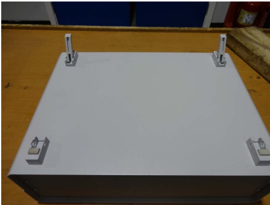
Figure 2.2.2 EUT 4. Enclosure with Case Feet canted ready for topple test
