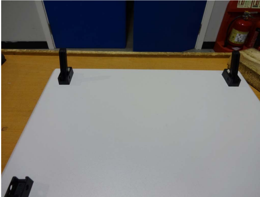
Figure 2.2.9 Post-Test Inspection. EUT 6. Case Feet. No damage observed to the feet or the enclosure
